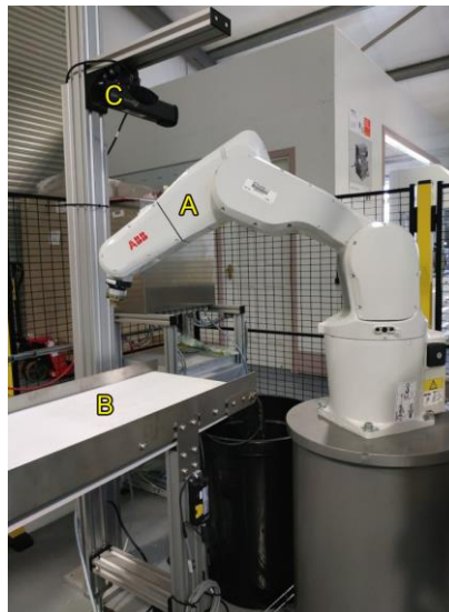
Figure 4 Robotic arm(A), conveyor belt(B), and Photoneo(C) of the pilot line
